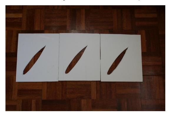
When placed together this gave enough depth for the float to sit comfortably in the foam board stack (expert advice has since told me the plane should be sitting higher in the water and the stabilising floats should be clear of the water).
