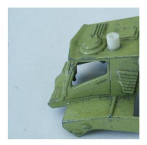
The next stage was to fix to roof doors in a permanently closed position, fill the gaps with Milliput and sand to give a smooth body.
